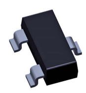
TopLine's series of SOT23 Jumpers withstand 75VDC at 100mA with 350mW power dissipation. Their operating temperature range from -65°C to +150°C. Standard and halogen free versions are available, and versions with up to 8 shorted pins are available. For more information, visit <a href="https://www.TopLine.tv/SOT23">www.TopLine.tv/SOT23</a> Jumper.pdf.
